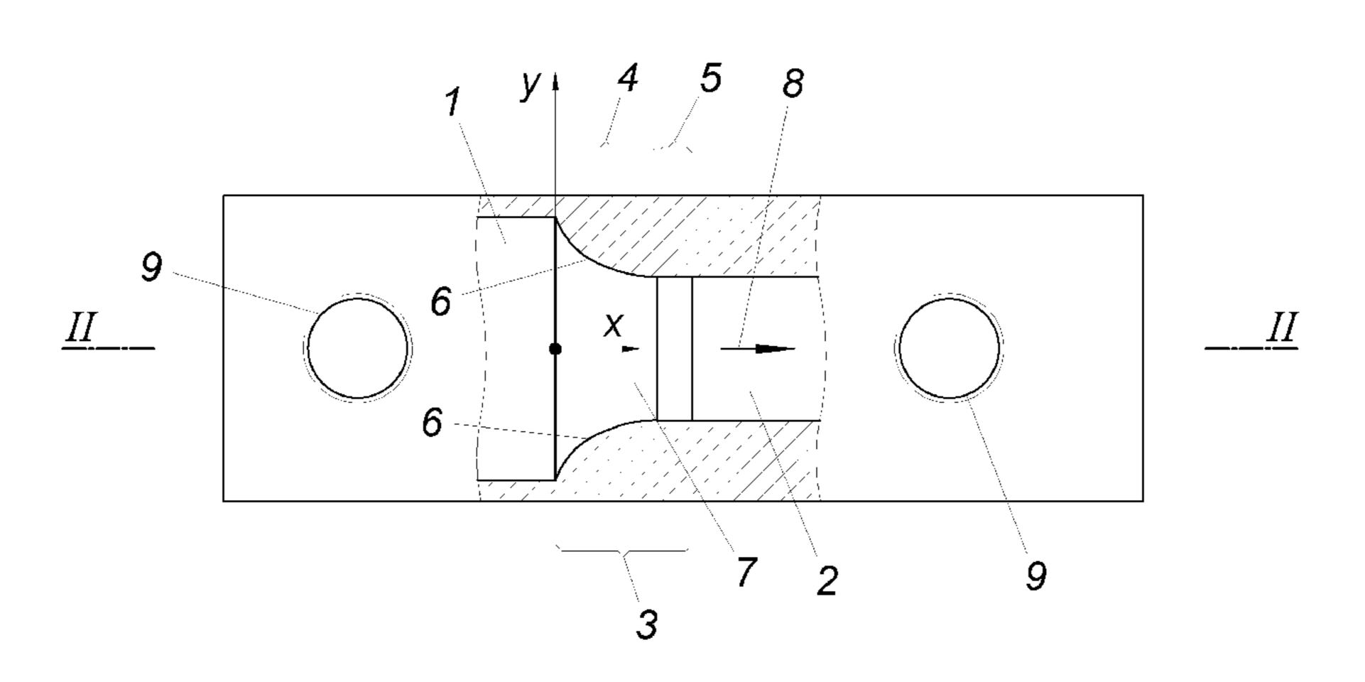
zone (5) which adjoins the inlet-side zone and in which two of the channel walls (6, 7) disposed opposite one another in pairs extend parallel to one another, while the two channel walls (7) arranged therebetween converge hyperbolically in the flow direction (8).
