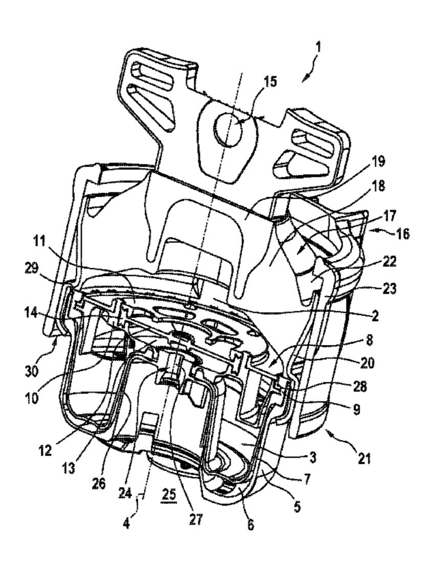
accommodates the fluid equilibration chamber, and a supporting part, which holds a spring element of the bearing system.
