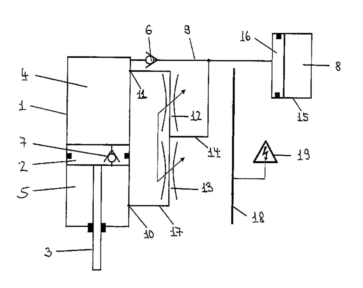
controllable operating valve (12) being provided between the compression chamber (4) and the rebound chamber (5).
