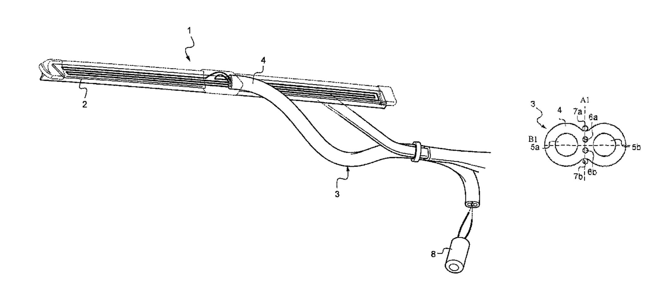
first spray line of the wiper blade, and the second circulation channel for the washer fluid is connected to said second spray line of the wiper blade.
