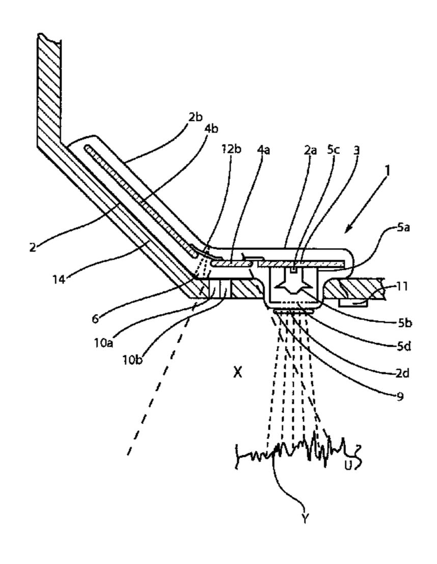
the control and evaluation device. The illumination device is adapted to be actuated by the control and evaluation device. A target area characterizing a detection area outside of the housing can be marked by an optical signal. The illumination device is adapted to be activated by the control and evaluation device for emitting light with different colors.
