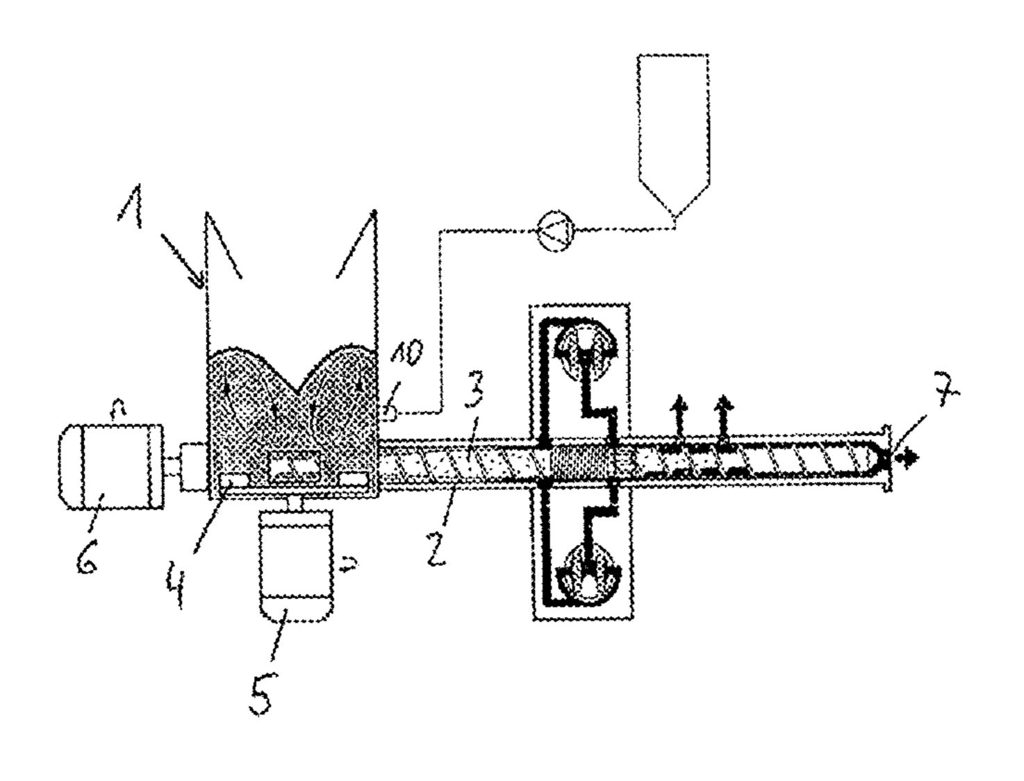
and mixed, and optionally warmed and reduced to small pieces in a receptacle and/or compressor, said material being in particular polymer particles and/or flakes, wood fibers, paper cuttings, or similar materials. According to the invention, the additive material is introduced below the level of the material and/or material particles already in the receptacle.
