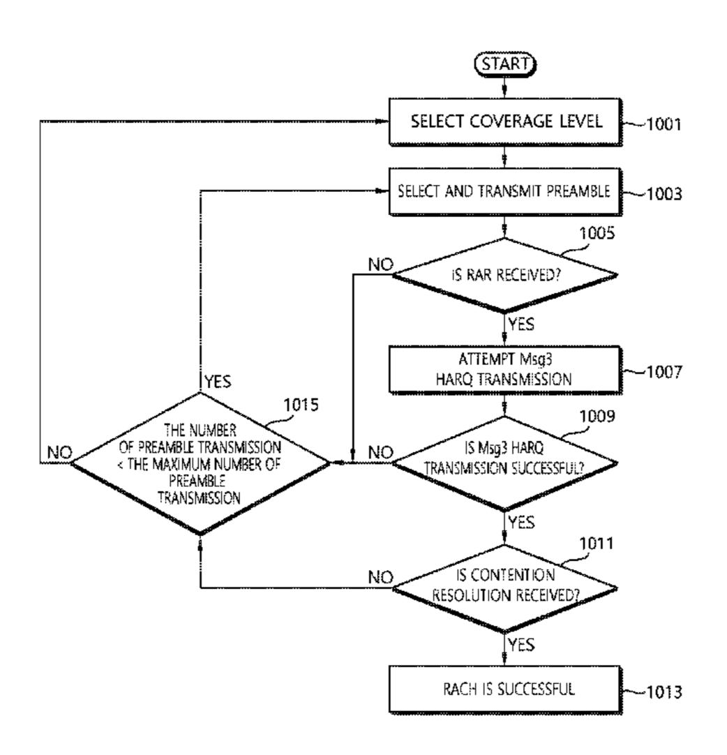
tion device which operates in cellular based IoT system perform random access, number of repetition may be increased, when coverage level is changed, by minimizing the change in coverage level, and operation time of the terminal, due to standing by up to PRACH resource corresponding to the coverage level, may be reduced to reduce energy consumption and to enhance delay time performance.
