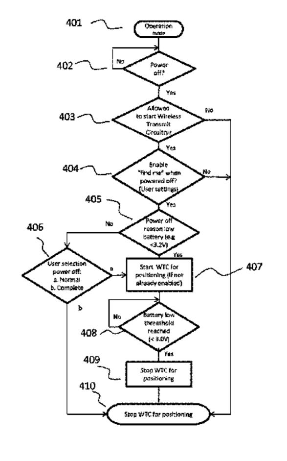
supply decreases below a threshold voltage, whereby the wireless circuitry will be broadcasting.
