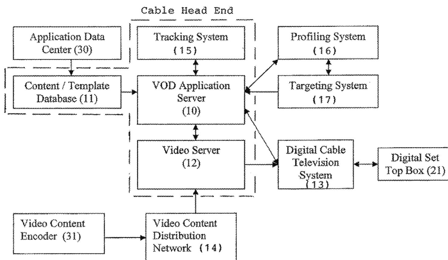
Figure 1A: VOD Content Delivery System, Overall Architecture
