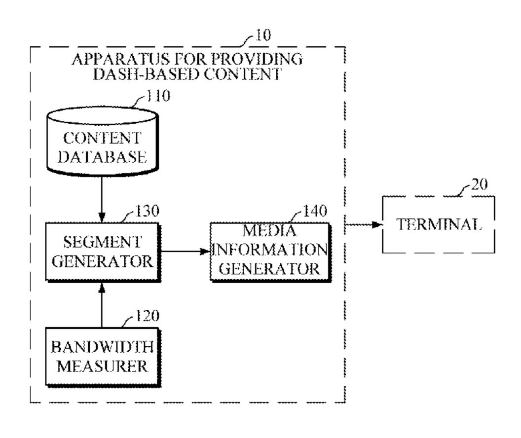
ith bandwidth itself among bandwidths of the network measured at the predetermined time intervals is increased or decreased by half of the predetermined bitrate difference, and generates a plurality of segments corresponding to the calculated lengths.
