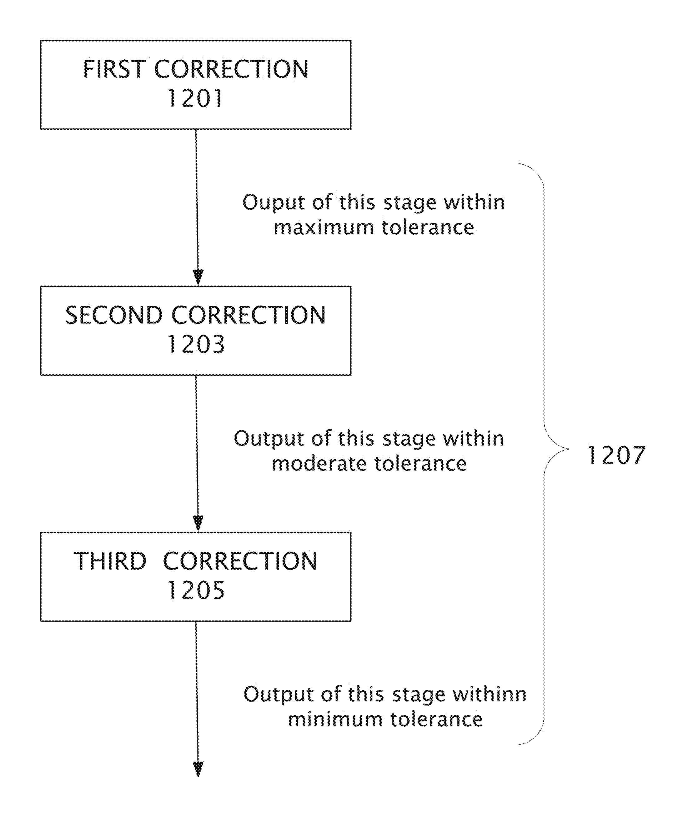
3 Stages providing required output 1200
