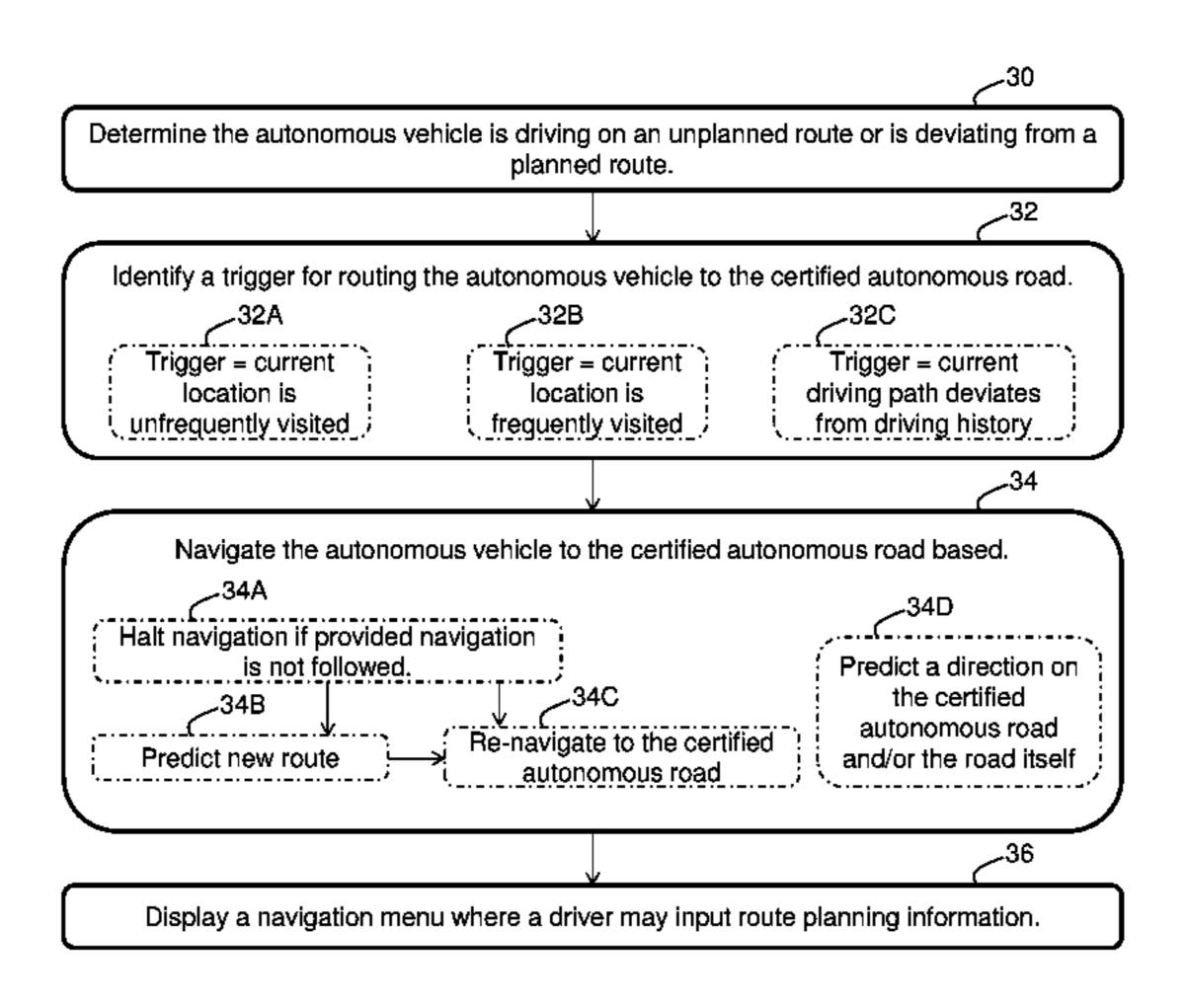
navigation unit only interacts with the driver once the vehicle is in the autonomous driving mode. The example embodiments have the advantage of providing navigation without requiring an interaction with a driver operating a vehicle in a manual driving mode.
