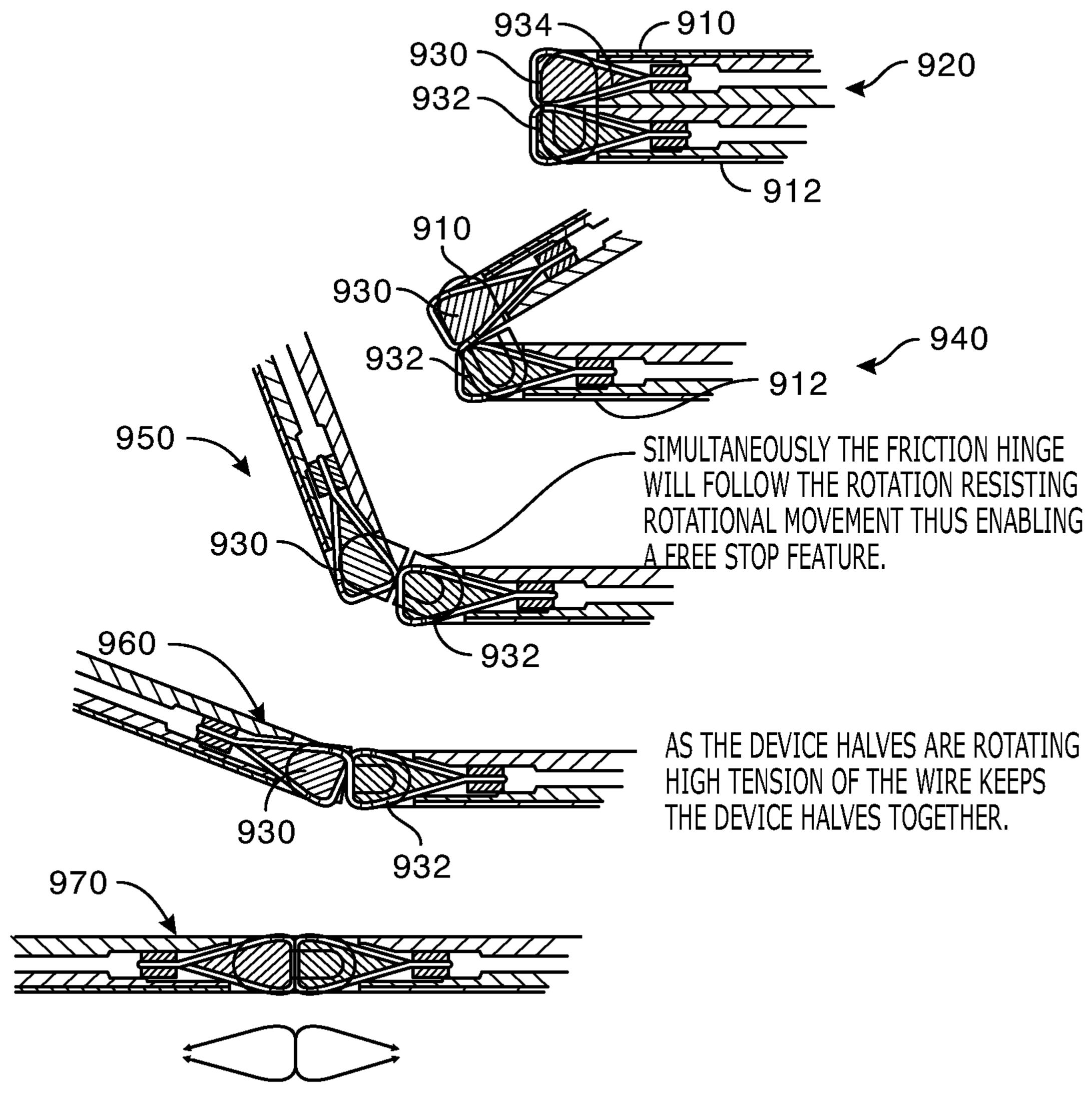
A WIRE LOOP IS TENSIONED AROUND HINGE LUGS. IN THIS CASE THERE ARE TWO LOOPS IN ORDER TO CREATE A BALANCED ASSEMBLY. EACH LOOP CREATES "A NUMBER 8 FIGURE".
