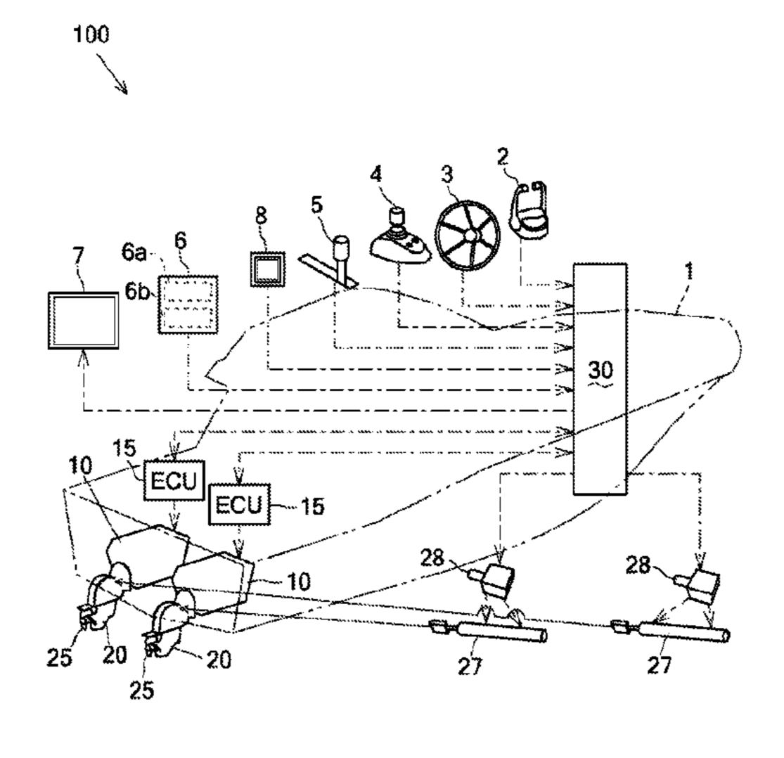
and speed exceeds a predetermined value, the ship steering control device corrects control values of the engine and the auto-drive unit.
