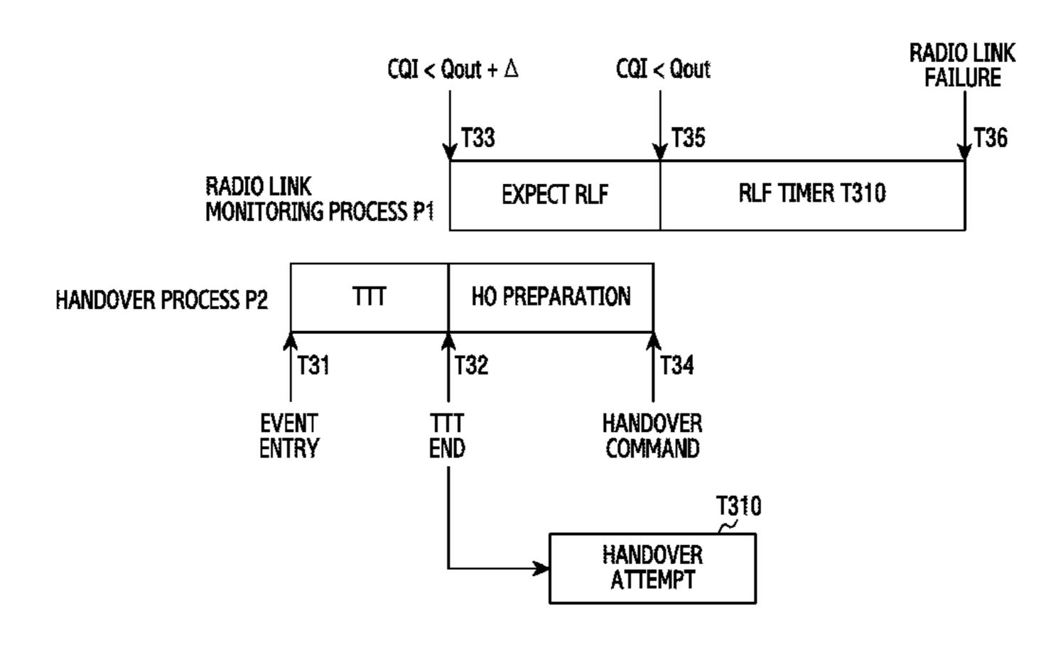
second timer regarding a radio link failure (RLF) is running, and if one of the first timer and the second timer expires, performing a radio resource control (RRC) connection reestablishment. When the handover and the RLF concurrently occur in the mobile communication system, the embodiments of the present disclosure can minimize the service interruption time by conducting the handover instead of the Radio Resource Control (RRC) connection re-establishment due to the RLF.
