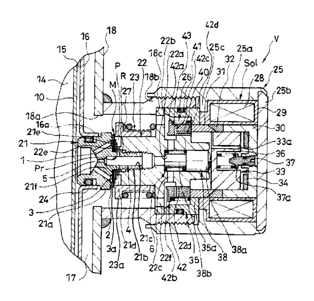
a valve opening pressure of the pilot valve. There is a time difference between a valve opening timing of the main valve and a valve opening timing of the pilot valve such that the valve opening timing of the main valve is delayed from the valve opening timing of the pilot valve.
