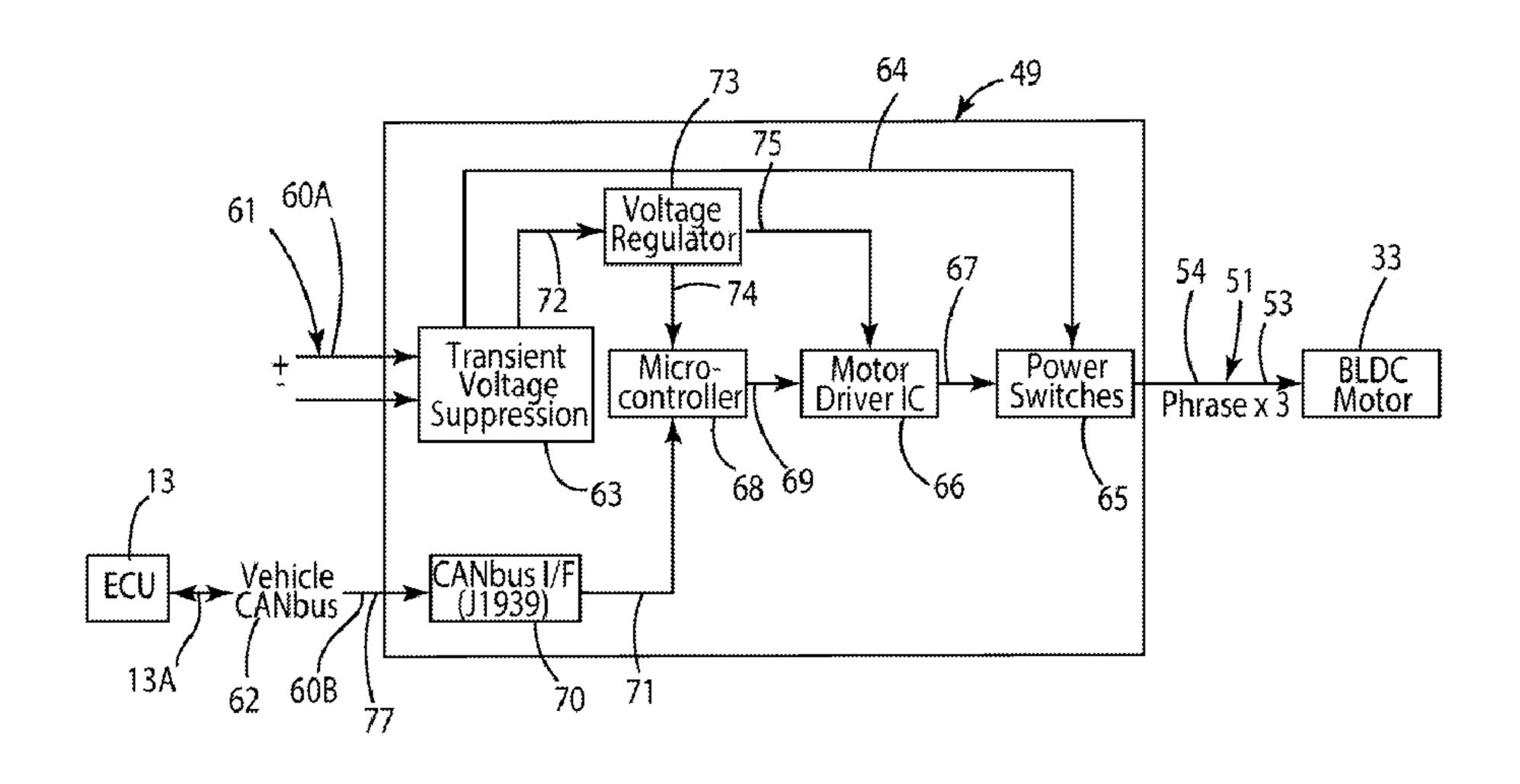
parameters of the motor to thereby provide a variable operate fuel pump.
