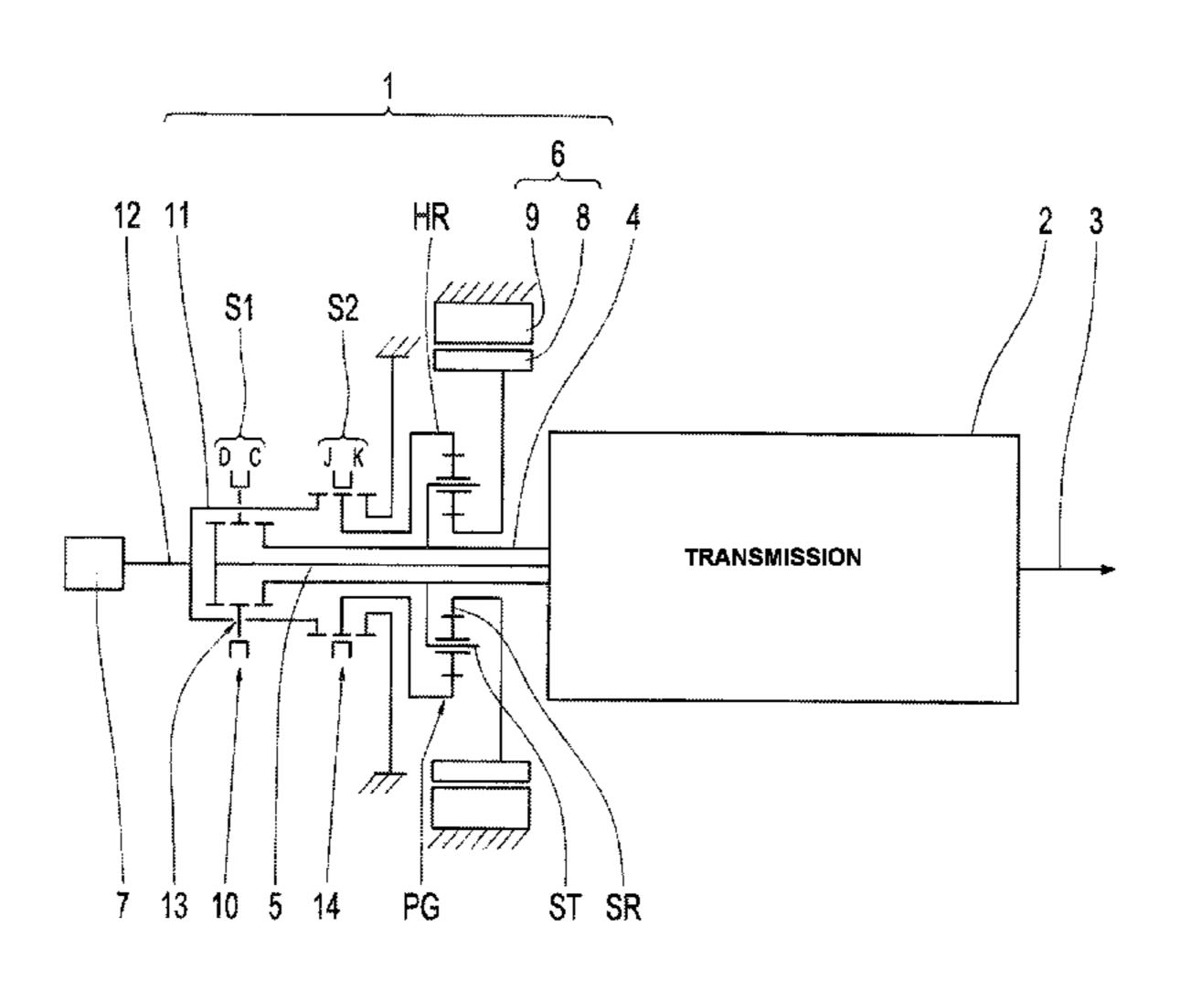
couples the third element of gearset (PG) with engine (7). Shift elements (C, D) respectively couple the shafts (4, 5) with engine (7) and form a double shift element (S1), whose actuator (10) extends through a section (11) of a drive shaft (12) of the engine (7), which encompasses, on the outside, shift element (S1). Section (11) of shaft (12) of engine (7) extends to shift element (J).
