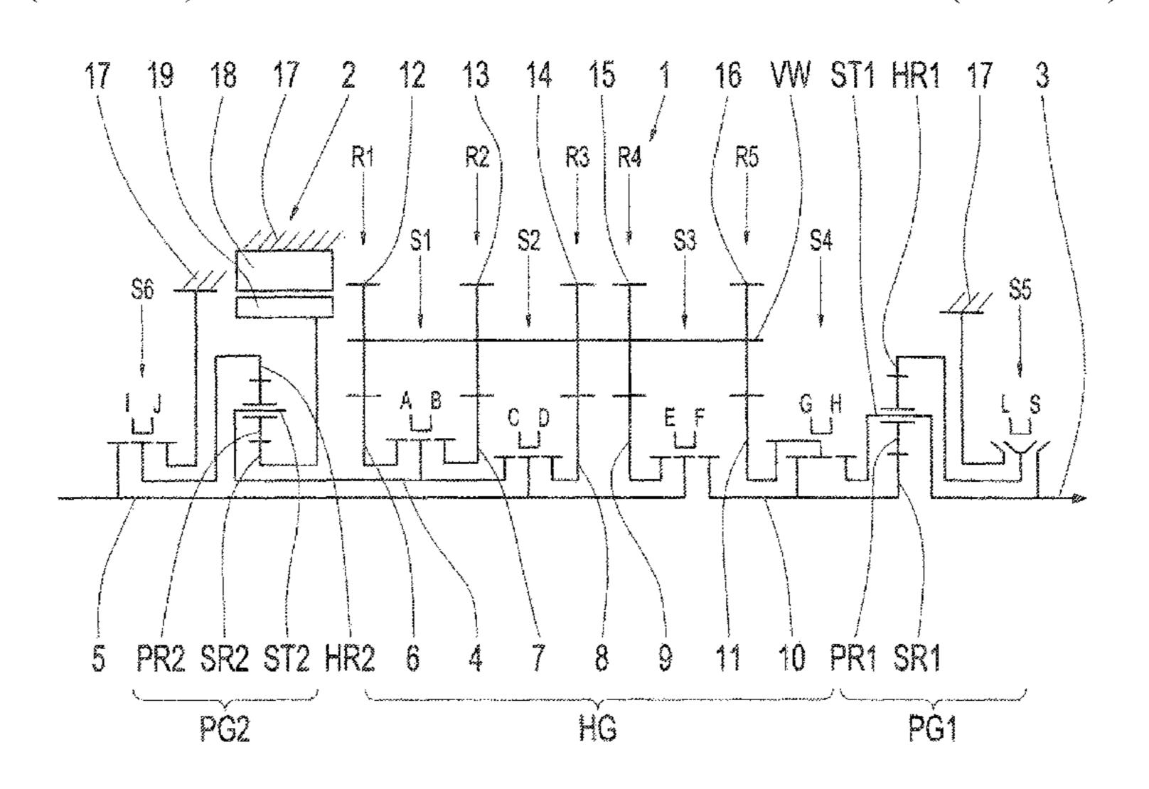
between an electric engine (2) and a first gear input shaft (4) of the main gear (HG). The fourth shifting element (S4), in a second shifting position (H), connects the fifth gear plane (R5) and the carrier (ST1) of the range group and thus the range group is able to be shifted under load.
