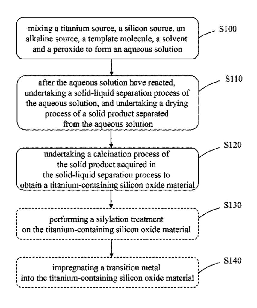
The titanium-containing silicon oxide material can be used to catalyze epoxidation of olefin and is very useful in epoxide production.
