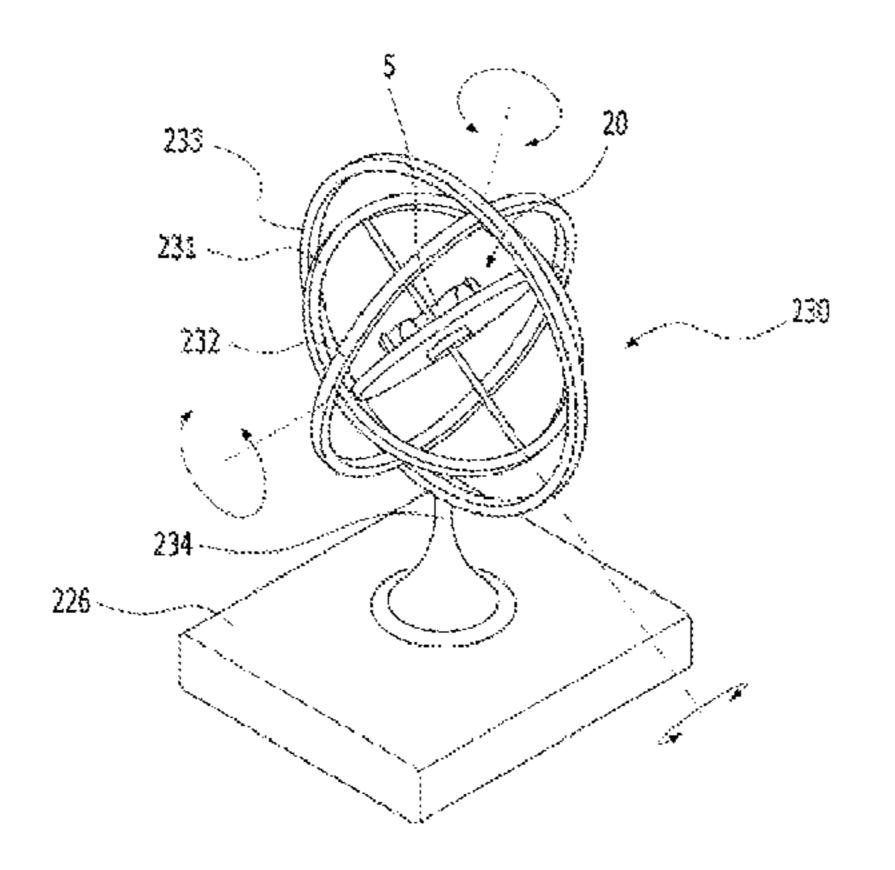
rotated about at least two axes with respect to an X-ray propagation path, wherein a CT image and high-precision three-dimensional surface data are reconstructed and provided by using a plurality of X-ray imaging data acquired through a plurality of scan sequences.
