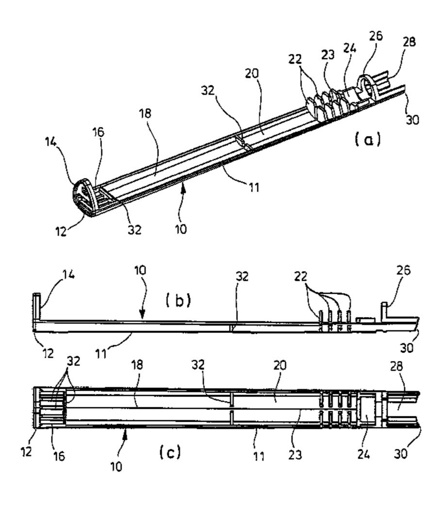
insert (10) permitting lateral access and fitting into the housing sleeve via one of the ends of the housing sleeve.
