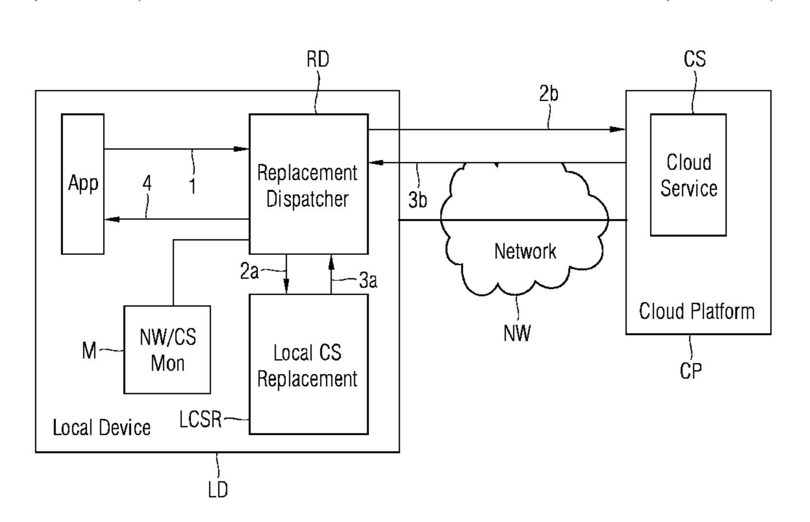
buffered, thereby cushioning connection interruptions between end device and cloud platform, whereby cloud services can be used in a transparent manner for the user and, even in the event of connection interruptions.
