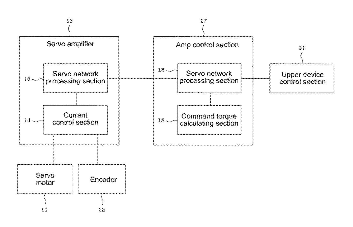
encoder without disconnecting the servo network when receiving the initialization instruction sent from the amp control section.
