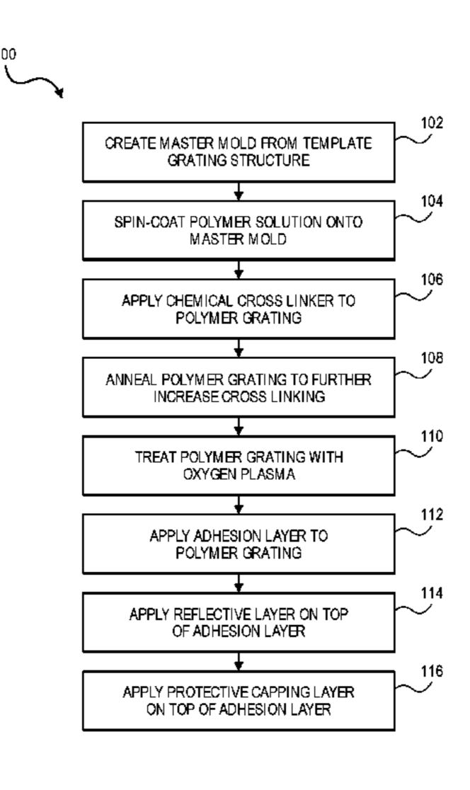
invention build nanograting structures layer-by-layer to optimize structural and optical properties and to enhance durability.
