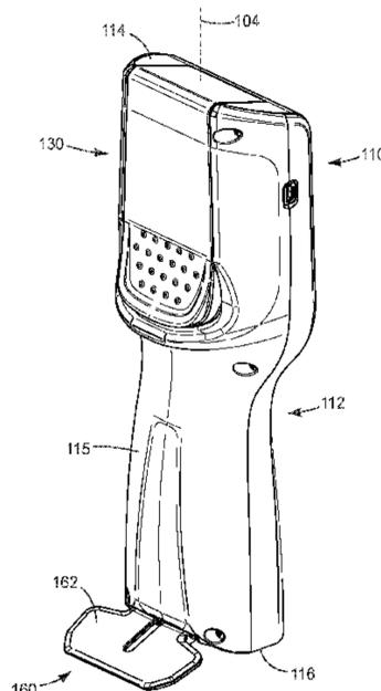
moved from a closed position to an open position. The support member is further adapted to maintain the light detection device in an upright position when the bottom surface and the support member are in contact with a working surface and the support member is in the open position.
