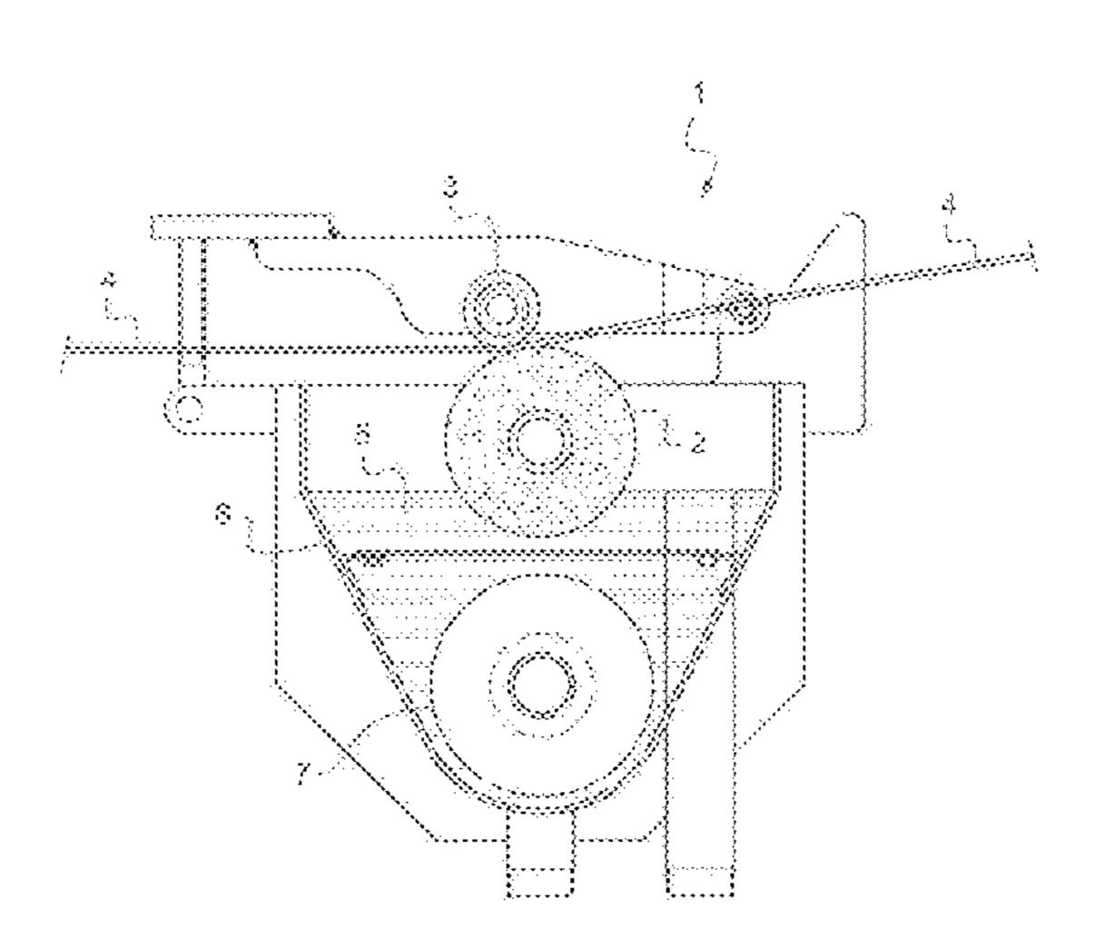
(4) is coated with the liquid composition including the fireproof additive using a roller.
