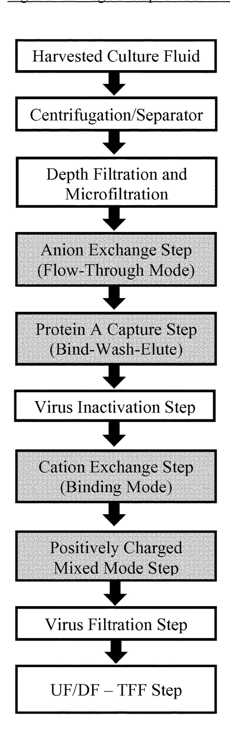
Figure 2: Exemplary process schemes of the invention using pre-cleaning steps
