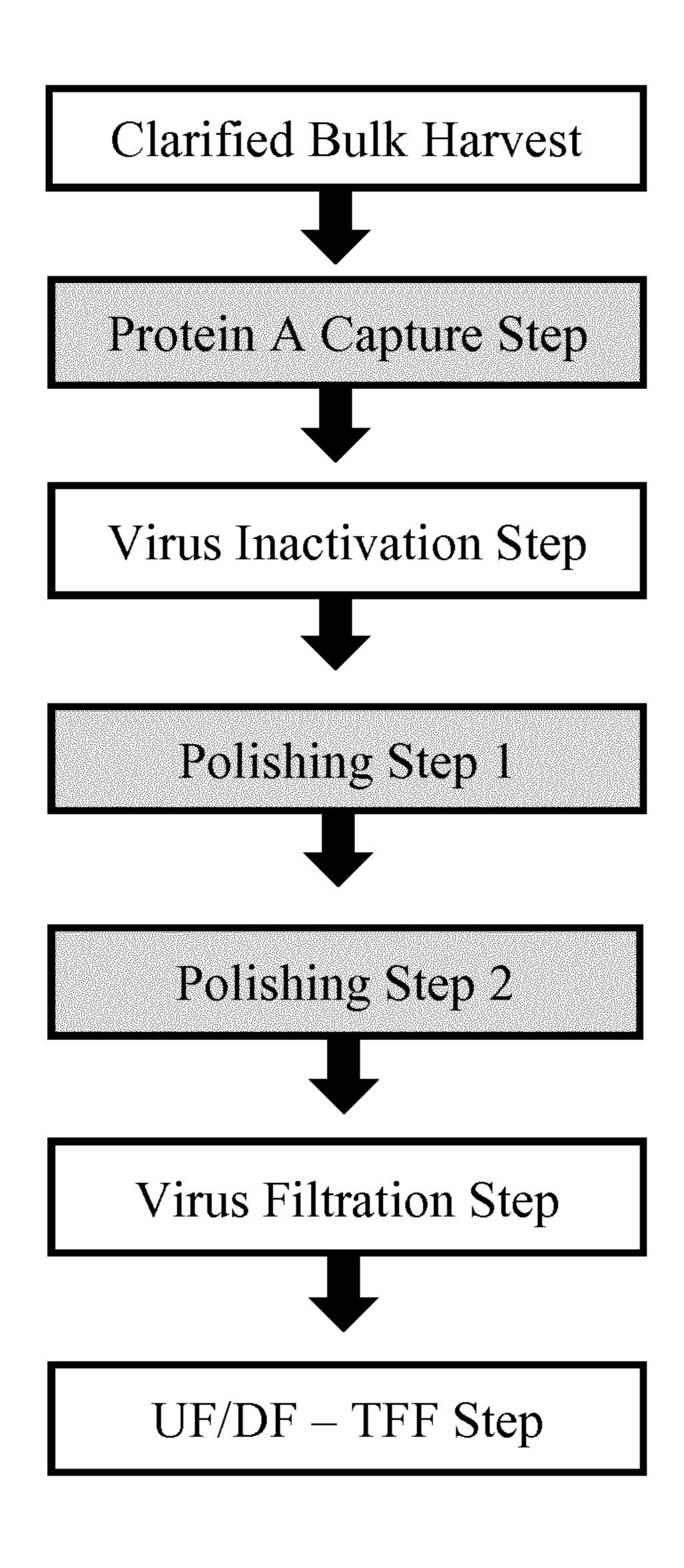
Figure 1: Process schemes of conventional purification methods for immunoglobulins
