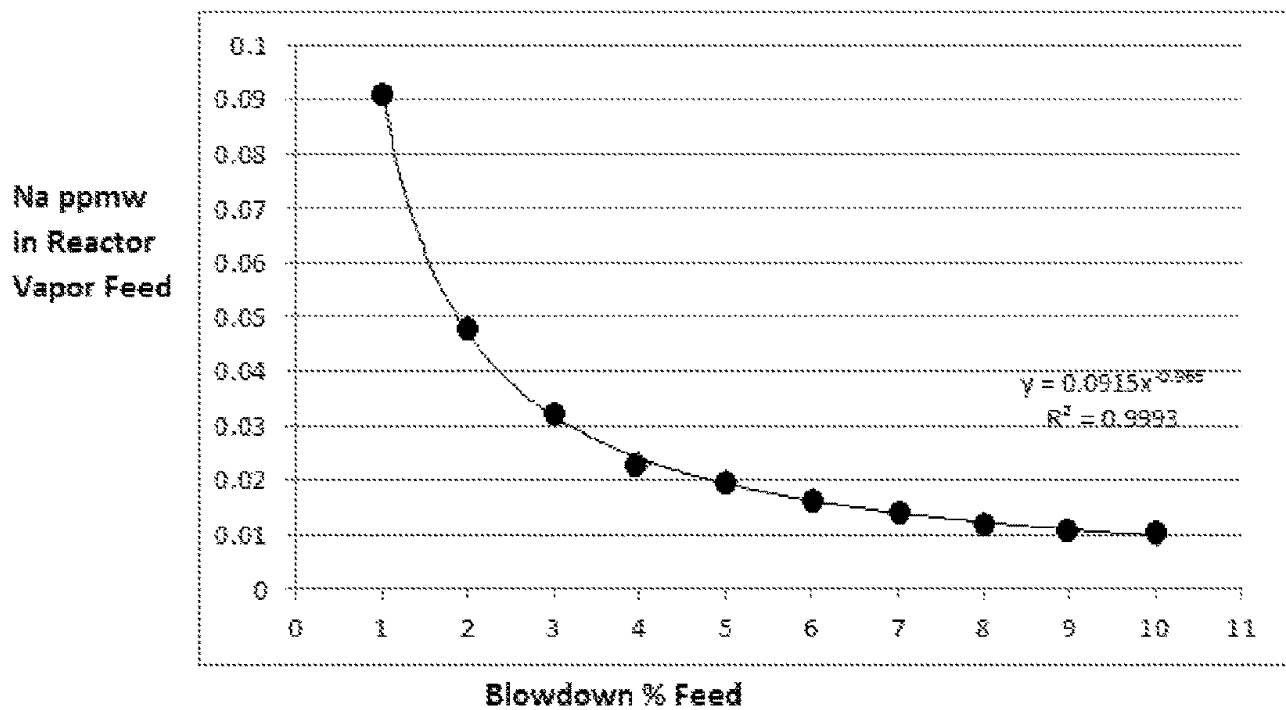
Figure 1-Feed Sodium with Blowdown from Methanol Vaporizer
