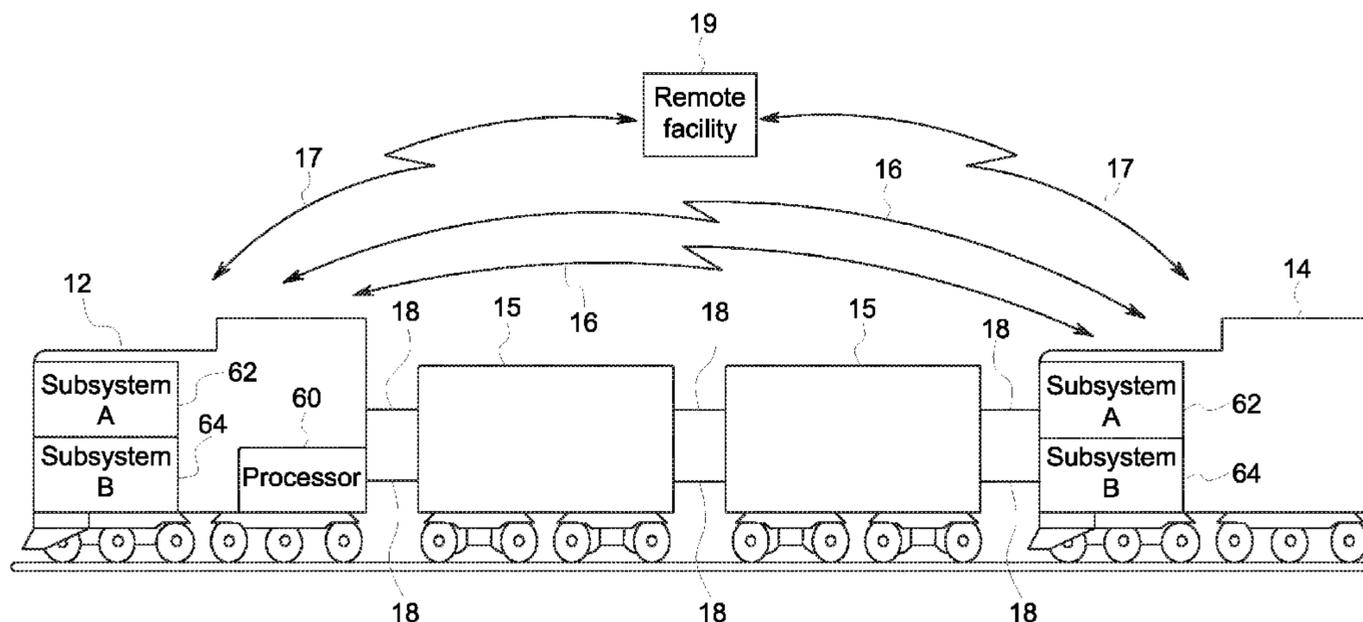
tional settings of the vehicle system at one or more different locations along a route being traveled by the vehicle system, different distances along the route being traveled by the vehicle system, and/or different times. The controller automatically changes the movement of the vehicle system according to the operational settings designated by the transitional plan to reduce the movement of the vehicle system to or below the operational restriction.
