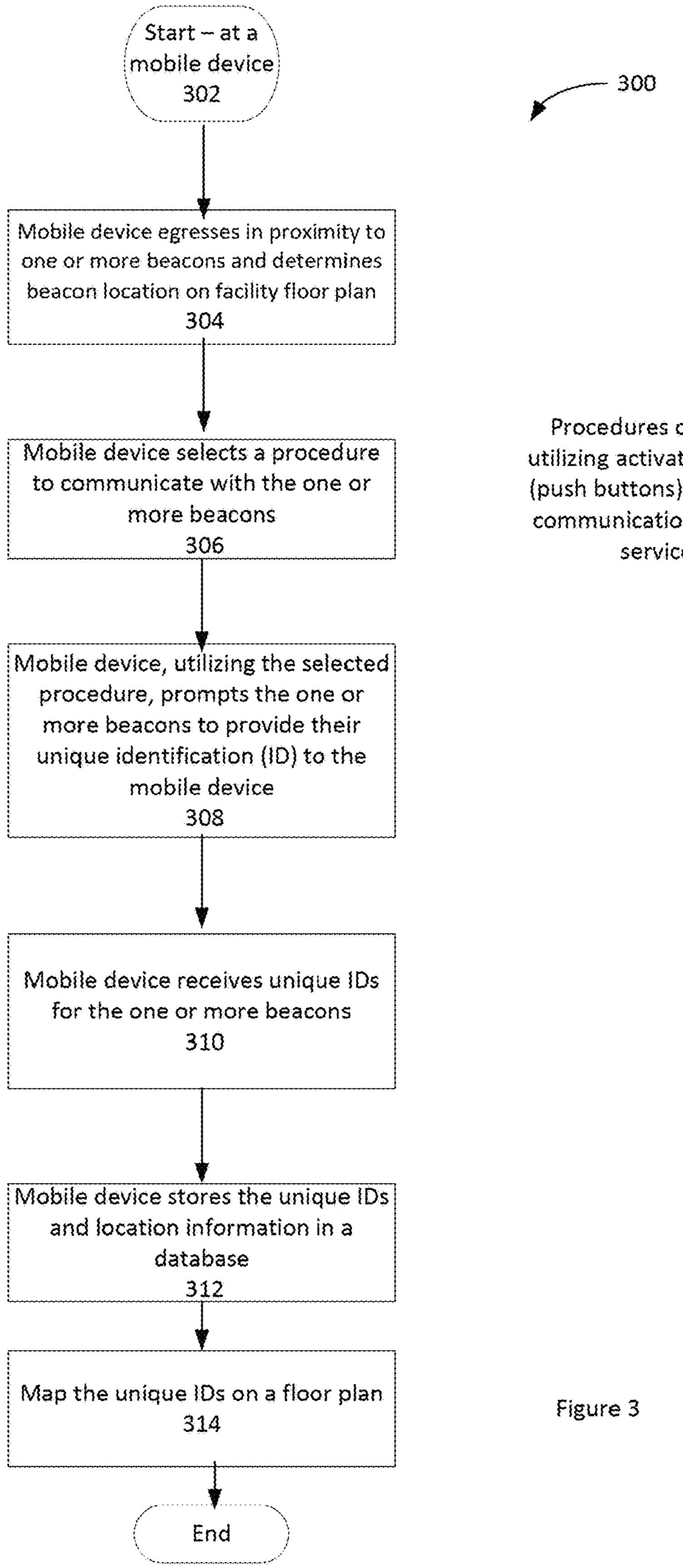
Procedures comprises utilizing activation sensors (push buttons) or wireless communication (BT GATT services)
