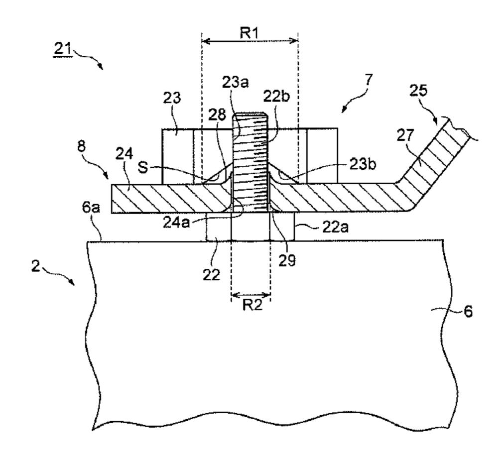
A flat portion of the bus bar is held between a bolt and a nut while the burr is located within a space created by the tapered portion.
