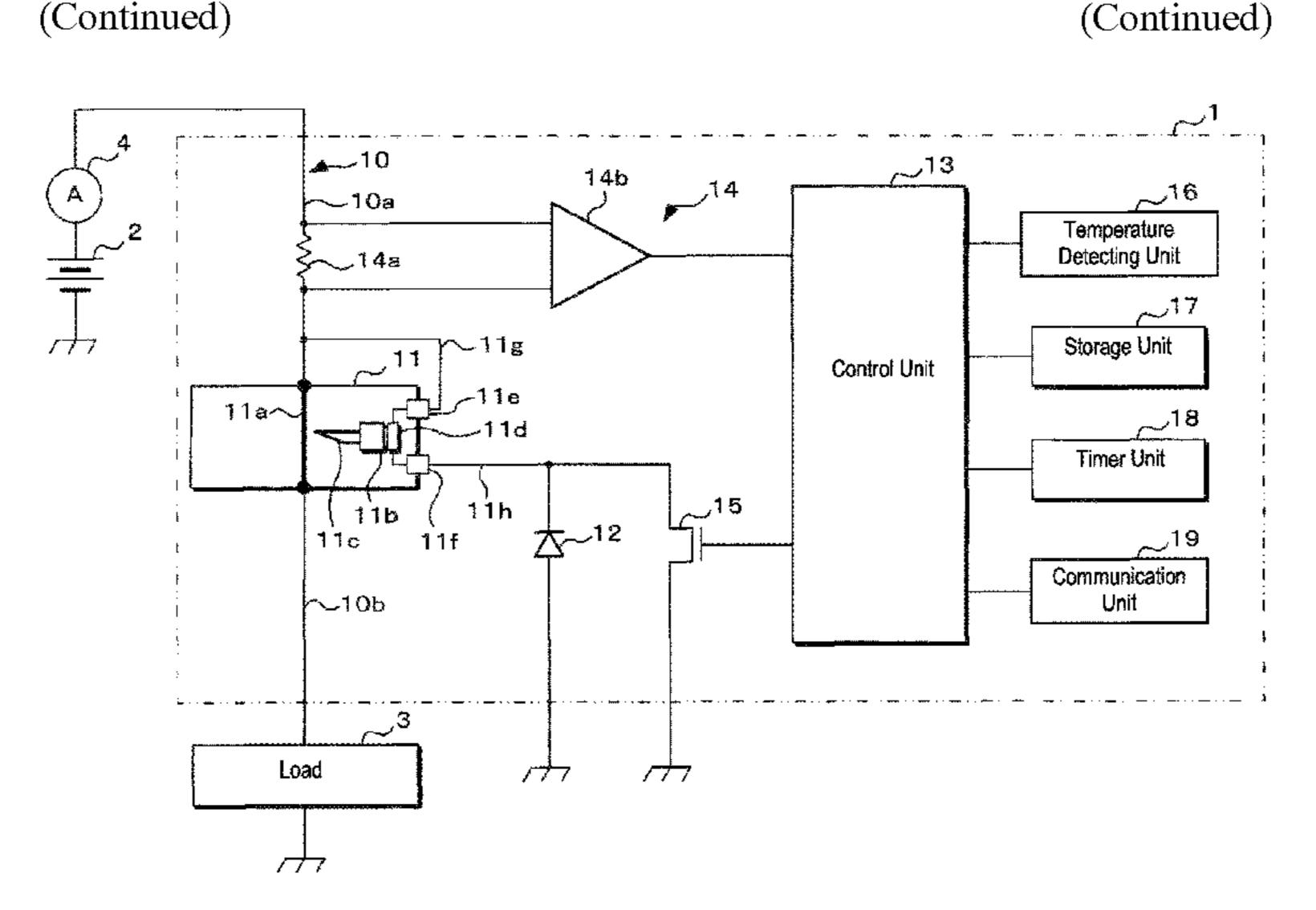
part is to be cut; and first and second terminals that input and output current that drives the drive part. In addition, the electric wire protection device comprises: a conductive wire having one end thereof connected to the electric wire and the other end thereof connected to the first terminal; and a diode having an anode connected to the reference potential and a cathode connected to the second terminal.
