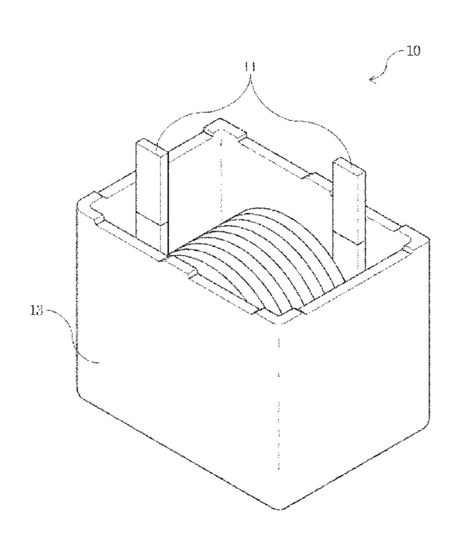
method is provided of a coil-embedded inductor having a structure in which a part of a coil is embedded in a magnetic core, which includes preparing an organic vehicle, preparing a soft magnetic molding solution having the density of 5.5 to 6.5 g/cc by mix-milling a soft magnetic powder with the organic vehicle, positioning and fixing a part of the coil in the case, and forming the magnetic core by injecting and curing the soft magnetic molding solution into the case.
