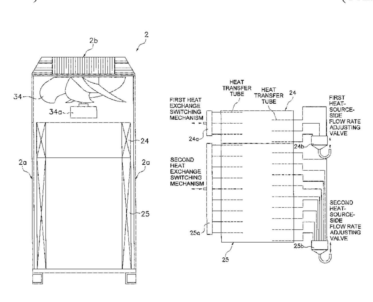
tively. In a defrost operation in order to defrost the first and second heat-source-side heat exchangers, the opening degrees of the first and second heat-source-side flow rate adjusting valves are controlled so as to achieve a defrost flow rate ratio at which more refrigerant flows to the second heat-source-side heat exchanger than during an air-cooling operation.
