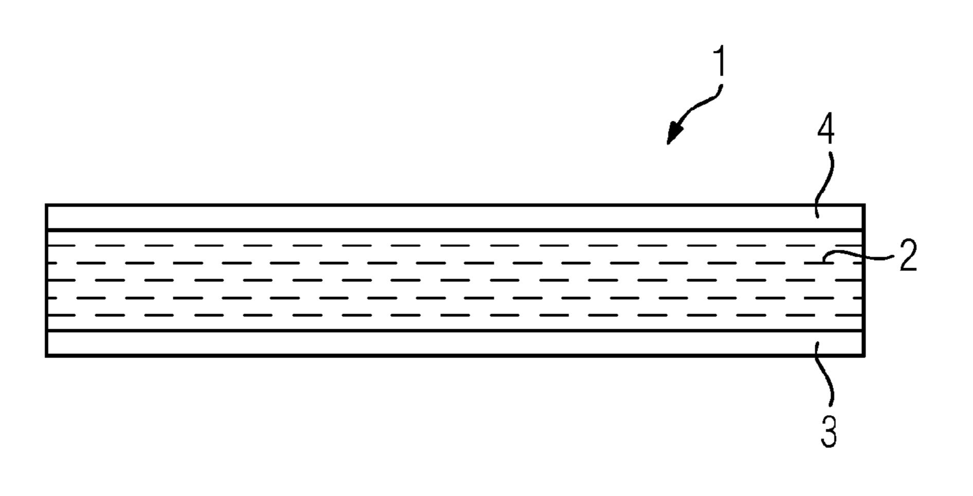
impregnating resin has an epoxy resin, a curing agent and nanoscale and/or microscale inorganic particles.
