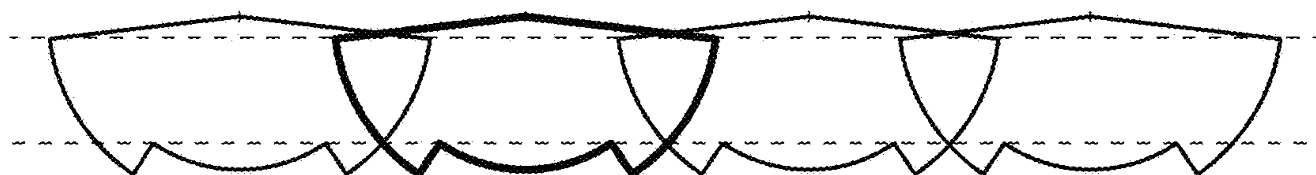
(a) Improvement bodies in a case where the jet grouting cannot be carried out from the top of a wall portion with an effective wall thickness.
