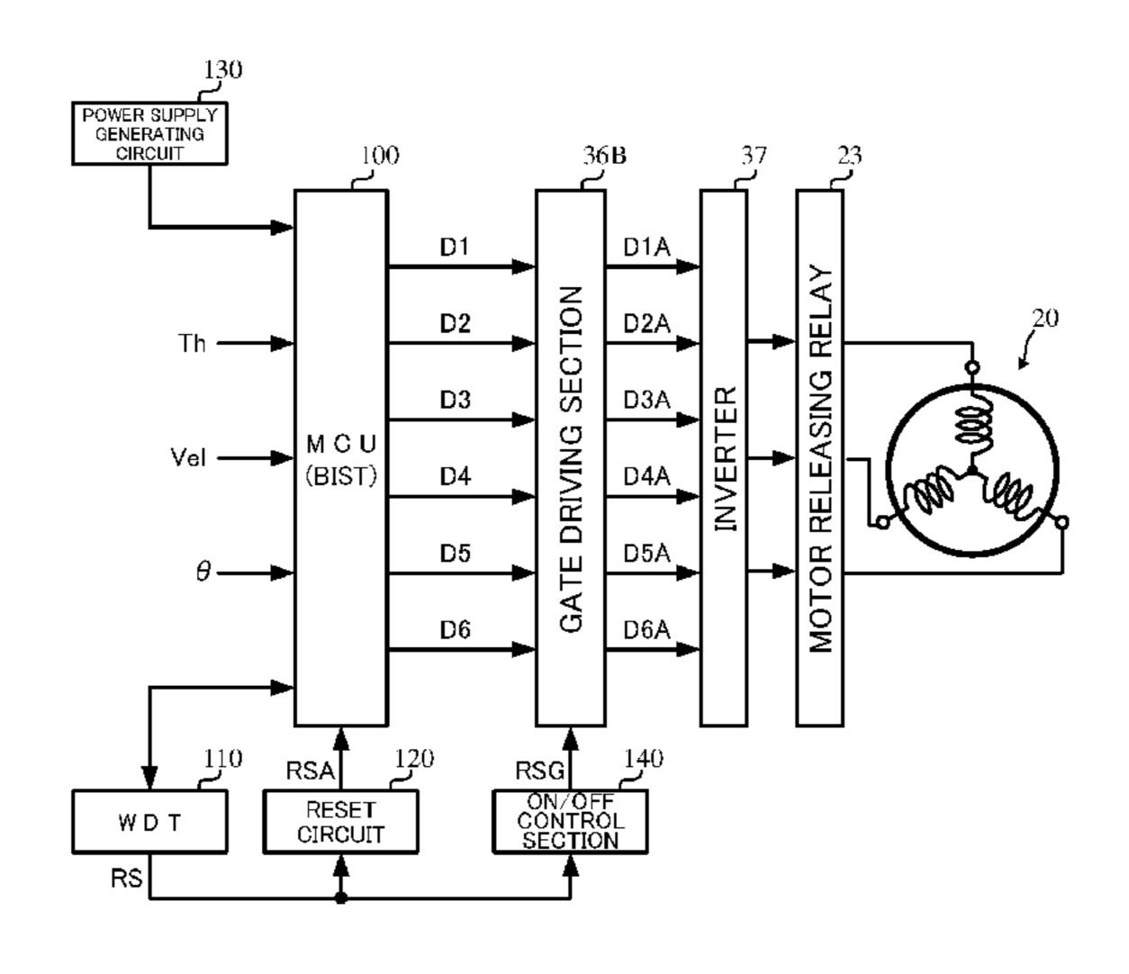
gate off via the ON/OFF control section when the external WDT is a disable state. When the abnormality of the MCU is not detected in an enable state, the inverter is driven by turning the gate on via the ON/OFF control section. When the abnormality of the MCU is detected, the inverter is stopped by turning the gate off via the ON/OFF control section and the MCU is reset by the reset circuit.
