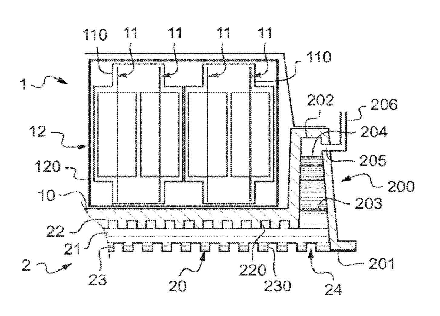
expansion vessel able to absorb the expansions of said phase-change material as it changes phase.
