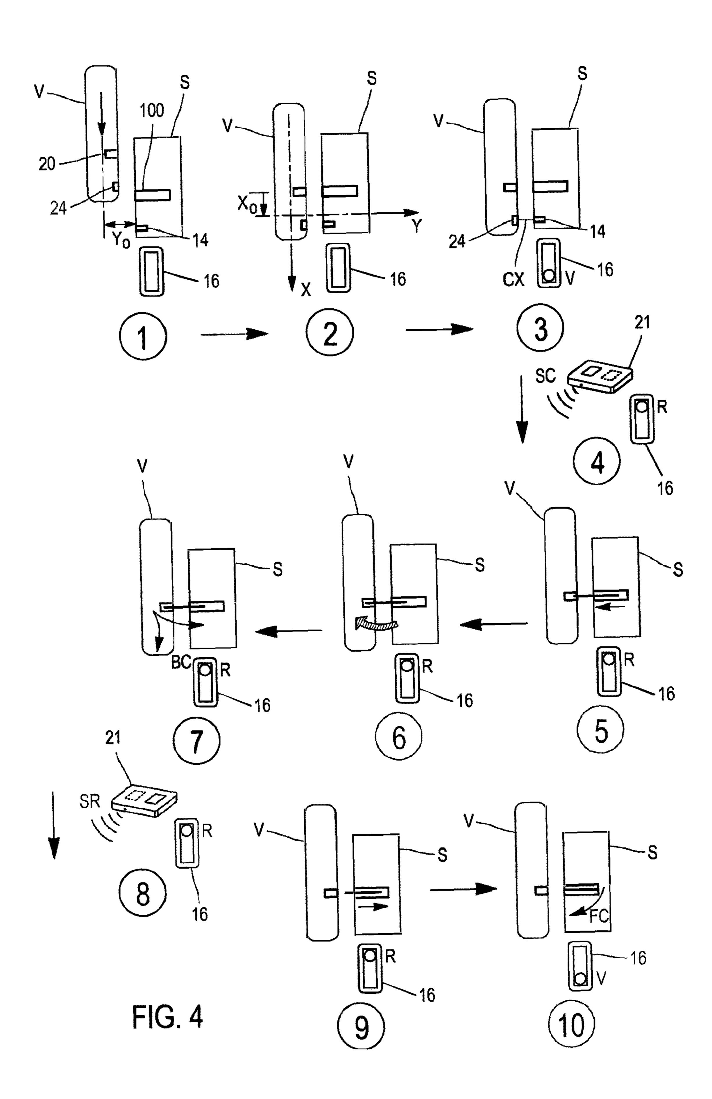
ASSISTANCE SYSTEM AND METHOD FOR THE POSITIONING OF AN ELECTRIC VEHICLE RELATIVE TO A CHARGING STATION, CHARGING STATION AND ELECTRIC VEHICLE IMPLEMENTING SAID METHOD
