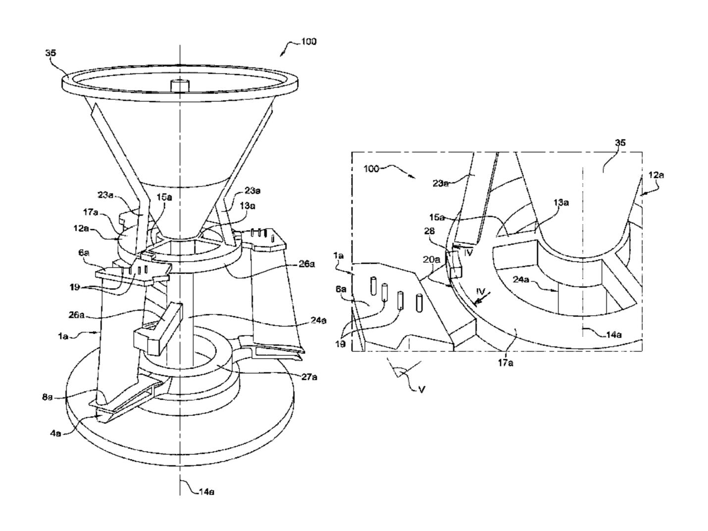
protective screen, associated with each second end portion and intended to protect a sensitive portion of the wire elements against the direct impact of a flow of metal from the feeder. The sensitive portion is located in the second end portion, downstream from the protective screen.
