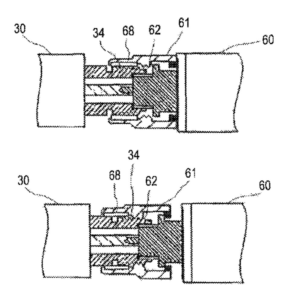
ment portion when the male-side connector is inserted into the female-side connector.
