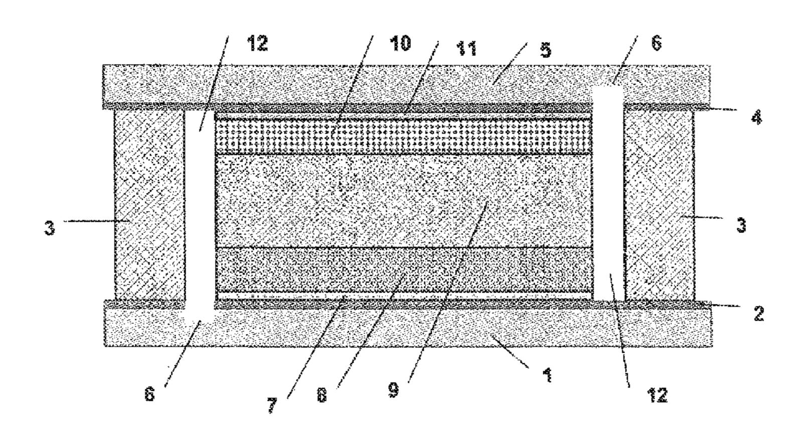
at least one photovoltaically active material which is introduced into the at least two porous carrier layers and has a concentration gradient.
