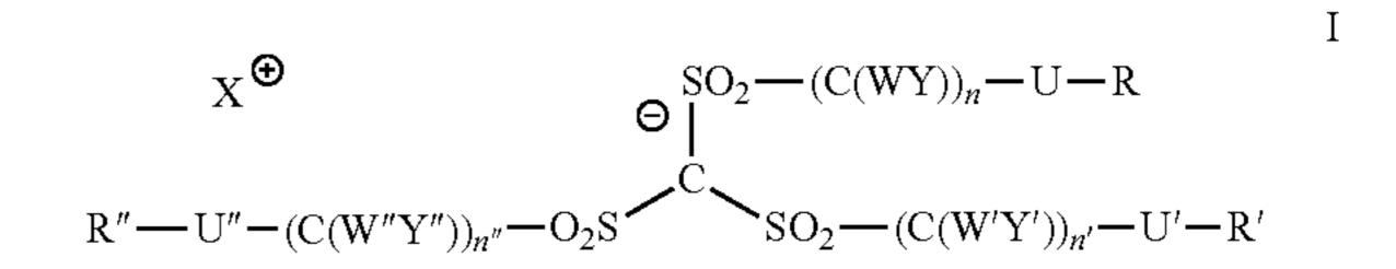
wherein W, Y are each independently hydrogen, fluorine, optionally substituted fluoroalkyl;
