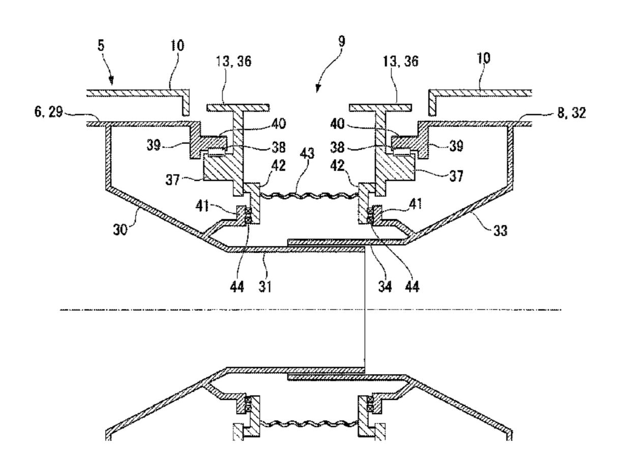
kiln inner cylinder. The externally heated carbonization furnace further includes a drive device that rotates at least one of the kiln inner cylinders and the kiln inner cylinder different from the at least one of the kiln inner cylinders and a control device that controls the drive device according to moisture content of a treated object in the kiln inner cylinder.
