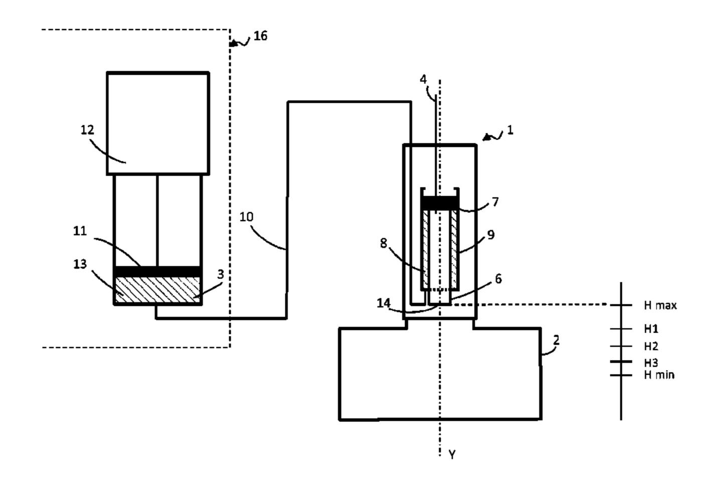
by suction of the movement transmission liquid into, or from the first chamber, the movement of the plunger tube, via the piston, into a first or a second direction, along the axis Y, for plunging into or moving upwards the fluidic circuit.
