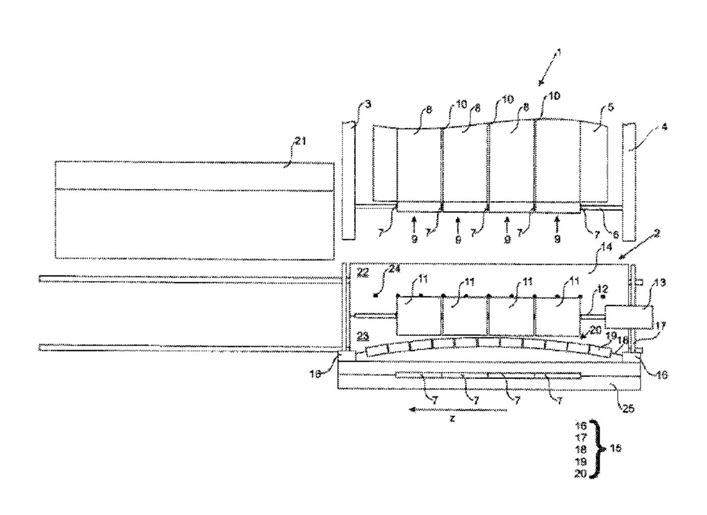
By means of this device for changing the position of the rolls axes, the roll axes of two adjacent rolls can be moved to an angle of less than 180 degrees in relation to one another.
