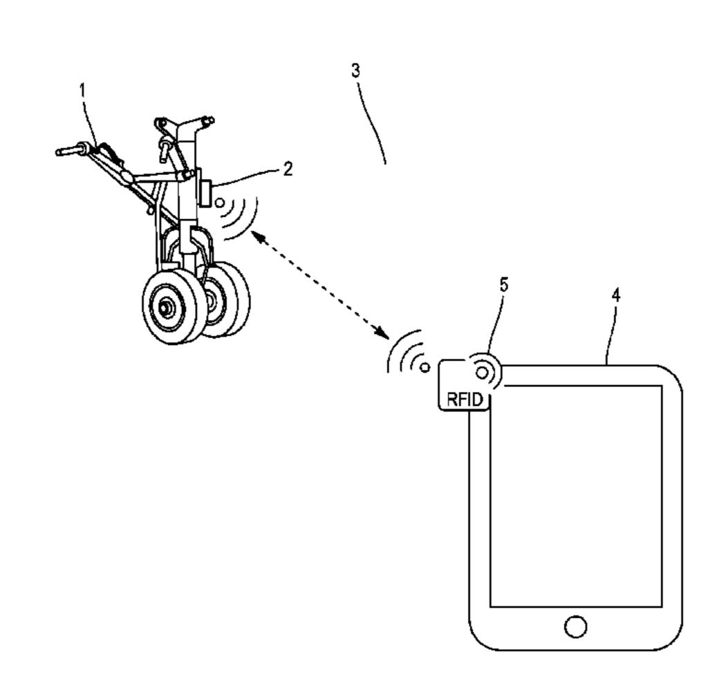
parameters relating to the ageing of the landing gear, and detecting a landing of the aircraft at a third sampling frequency until a predetermined period has expired. The third frequency is greater than the second frequency, which is greater than the first frequency. Measurements relating to the ageing are stored as a function of the measured physical parameters.
