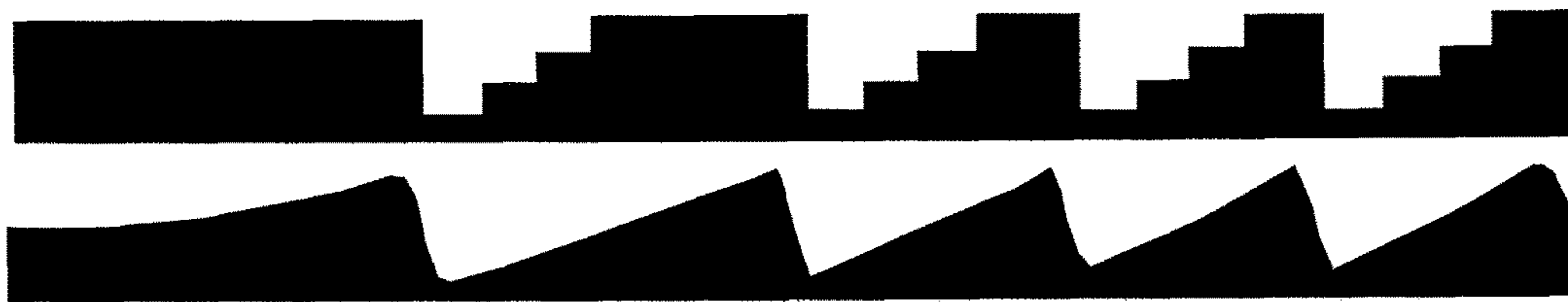
Schematic profile of an FZP with five zones and four steps and schematic profile of the equivalent modified FZR
