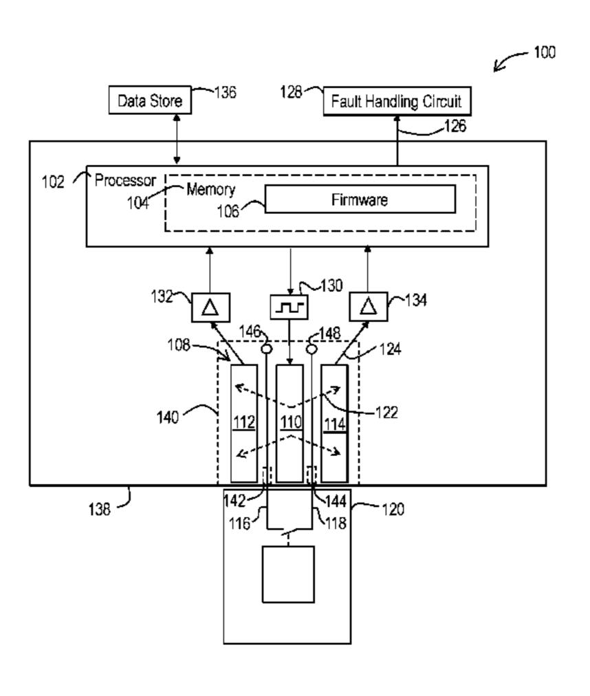
signal antennas, and responsive thereto output at least one communication (126) indicative of a fault with the relay being detected.
